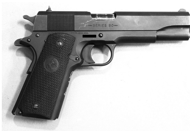
Figure 4.54 The Colt Model 1911 Series 80 chambered in .45 ACP. The Series 80 was manufactured from 1983 to 1988. Overtly, there is nothing different about the Series 80 from other 1911 pistols save for the introduction of an internal firing pin safety. Regardless of the manufacturer and exact date of manufacture, the 1911 design is classic and immediately recognized. (Image from author's collection.)
